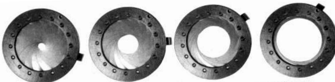
The iris diaphragm alters the size of the aperture and therefore the brightness of light reaching the film. Small apertures—f22 and f16—cut down brightness
